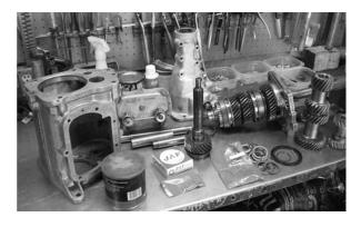
Muncie 4 speed transmissions rebuilt for \$275.00 labor, parts extra. The basic rebuild kit consists of front and rear bearings, all needle bearings, gaskets, snap rings, seals, synchro rings, front input retainer nut, synchro keys and springs. Also includes new counter shaft. My cost on the overhaul parts kit is \$126.00 plus shipping. Additional parts, if needed, are at additional cost.
